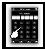
Press the hidden button Prog to exit the Settings Menu. Note: RFTC-10/G returns from the setup menu to the basic display automatically 30s after the last pressing of the button.
